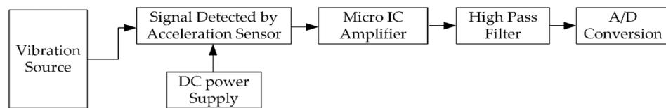
**Figure 2.** Acceleration signal processing diagram.
