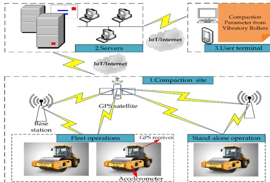
**Figure 1.** Overall framework of compaction operation monitoring system for an intelligent roller based on Internet of Things.
