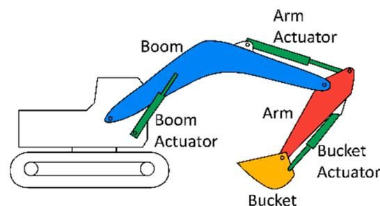
**Figure 1.** Hydraulic excavator and its main components.
