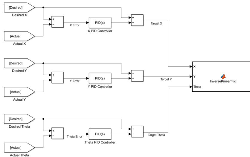
**Figure 5.** Schematic of contour error compensation.
