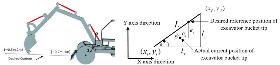
**Figure 4.** An example for the desired trajectory (contour) of a bucket tip (left) and the contour error (right) [3].
