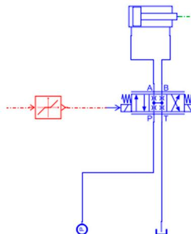
**Figure 2.** Hydraulic circuit of one cylinder modeled in Amesim software.
