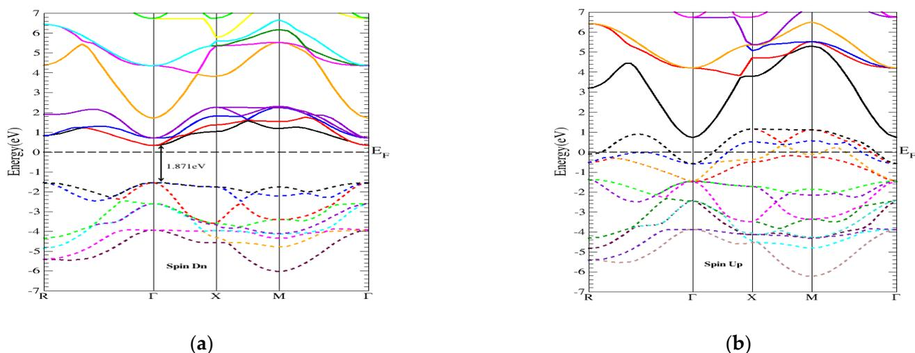
**Figure 2.** The NbScO<sub>3</sub> electronic band structures for (a) the minority (Spin Dn) and (b) the majority (Spin Up) channels with PBE-GGA.
