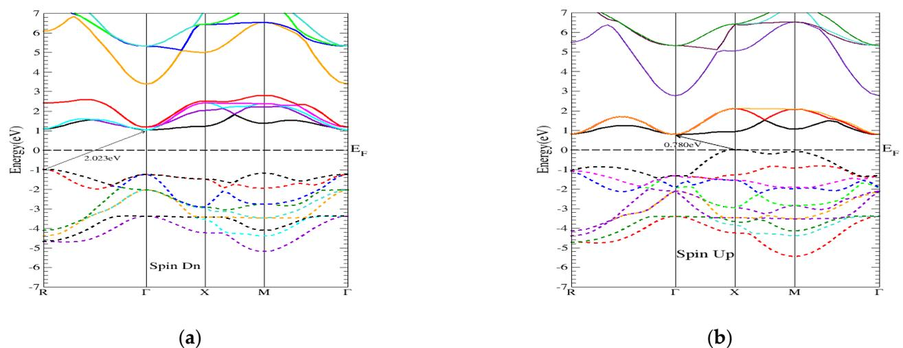
**Figure 3.** The NbScO<sub>3</sub> electronic band structures for (a) the minority (Spin Dn) and (b) the majority (Spin Up) channels with mBJ.
