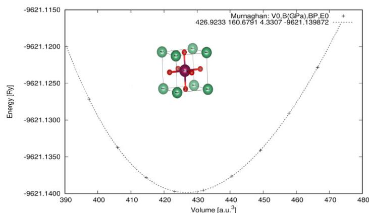
**Figure 1.** The energy-volume optimization and Murnaghan fit for the perovskite NbScO<sub>3</sub>.
