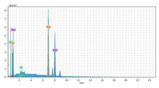
Figure 3. EDX analysis of the prepared product.
