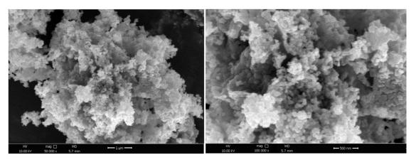
Figure 4. SEM images of resulting CuCo<sub>2</sub>S<sub>4</sub>/CuCo<sub>2</sub>O<sub>4</sub> heterostructure.
