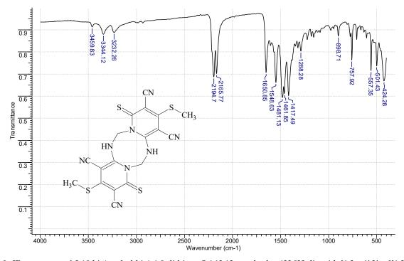
**Figure 2.** IR spectrum of 3,10-bis(methylthio)-1,8-dithioxo-5,6,12,13-tetrahydro-1H,8H-dipyrido[1,2-a;1',2'-e][1,3,5,7]tetrazocine-2,4,9,11-tetracarbonitrile ( $\mathbf{4}$ ; R = CH<sub>3</sub>, X = S).
