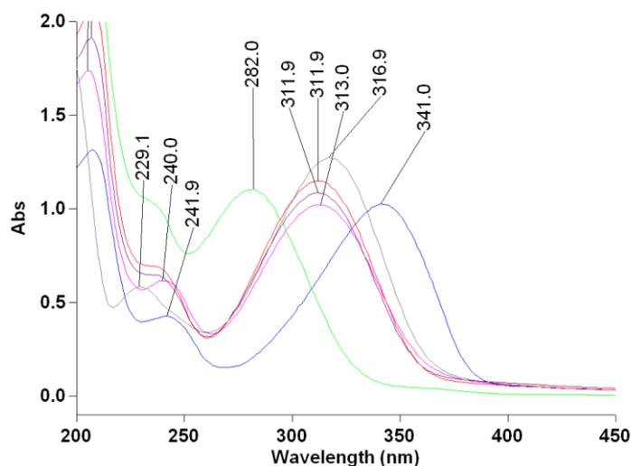
**Figure 3.** UV-Vis spectra in acetonitrile of symmetrical 2-bromobenzylidene MACs. **2BrCP** (blue line) **2-BrCX** (violet line), **4tB2BrCX** (red), **2BrCH(ep)** (green line), **2-Br4PIP** (pink line), and **2F4PIP (EF24)**, gray line).
