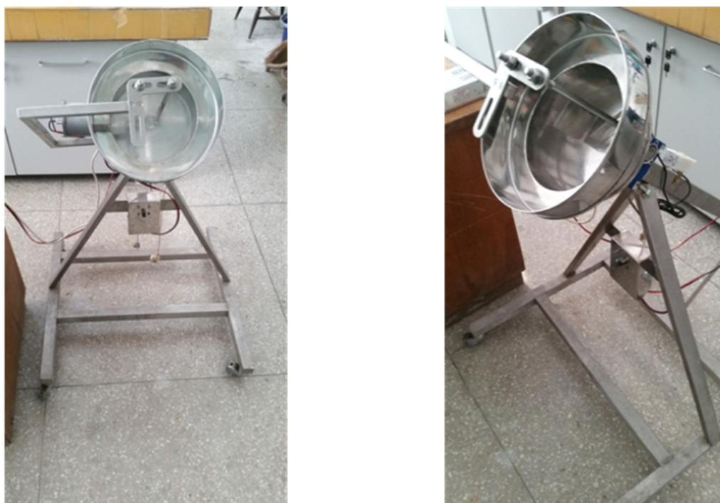
**Figure 1.** Custom-made rotating pan granulator developed in this study and used for granulation experiments.
