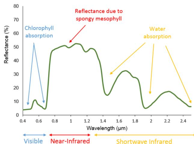
**Figure 1.** Vegetative spectral reflectance curve.
