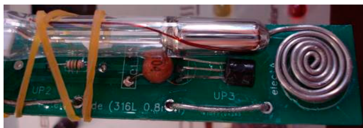
Figure 6. Assembly of the Hg thermometer on the IC, adopted for the temperature calibration.
