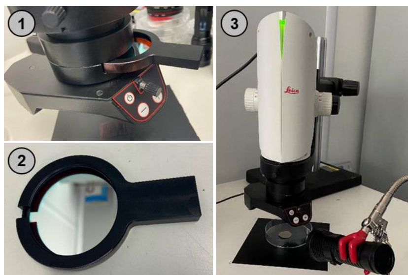
Figure 1. Modified digital microscope for fluorescent imaging. (1) Mounting bracket for emission filters. (2) Emission filter in holder. (3) Modified digital microscope with emission filter mounting bracket and LED flashlight.
