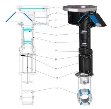
**Figure 4.** Section view of the optics system consisting of the vacuum window (1), optics holder (2), side closure (3), folding mirrors (4), objective (5), objective holder (6), rotating unit (7), fiber plate (8), fiber plate holder (9), optical fibers (10), and the fiber bundle holder (11).
