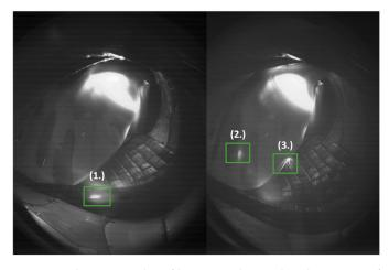
**Figure 1.** Three examples of hot-spots detected in the images of the visible video diagnostics. (1.) A hot-spot on the shielding of the magnetic diagnostics, created by the misconfiguration of the magnetic field structure. (2.) A hot-spot on the reciprocating probe. (3.) A hot-spot made from debris falling into the vessel.
