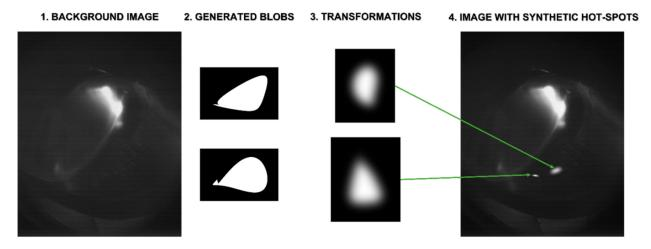
Figure 3. The steps in the process of generating images with synthetic hot-spots.
