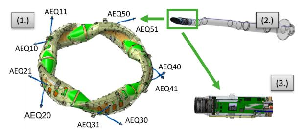
**Figure 2.** (1.) Overview of the visible video diagnostics ports in the vessel. (2.) One of the AEQ ports is connected with a flexible tube. (3.) A camera head containing only the most important electronics and optics.
