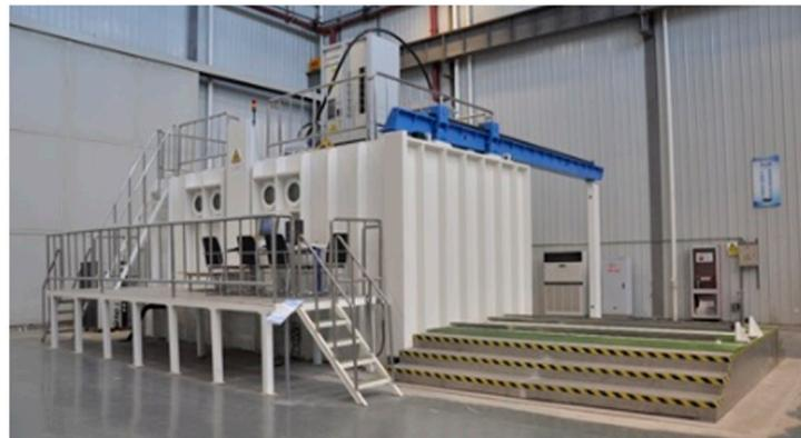
Figure 2. The experimental equipment of electron beam welding (EBW).
