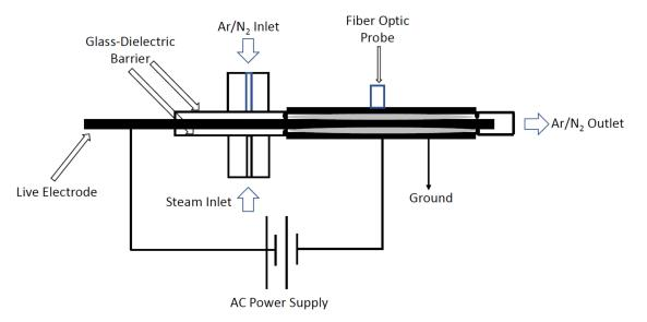
Figure 3. A simple DBD-corona reactor.
