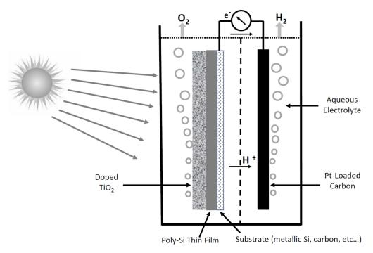
Figure 2. Solar water splitting system using a composite semiconductor electrode.
