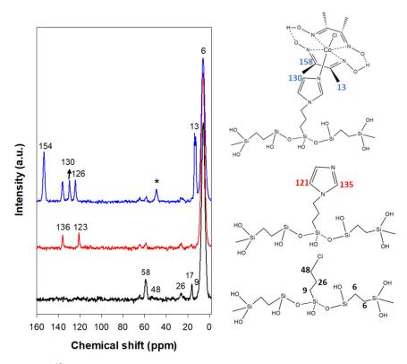
**Figure 4.** <sup>13</sup>C CP/MAS NMR spectra of Cl-EtPMO (black line), Im-EtPMO (red line), and Im-EtPMO-Co (blue line). Predicted chemical shifts on the right. \*—low field.
