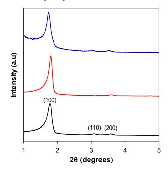
Figure 1. PXRD of Cl-EtPMO (black line), Im-EtPMO (red line), and Im-EtPMO-Co (blue line).
