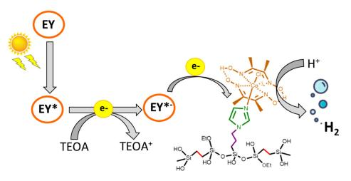
**Scheme 2.** Schematic representation of photocatalytic hydrogen evolution reaction with TEOA and Eosin Y (EY) as electron donor and photosensitizer, respectively. (EY\*, photoexcited EY).
