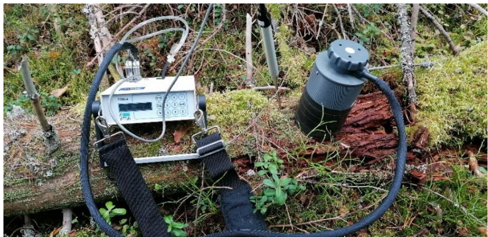
Figure 8. Portable infrared gas analyzer operating in closed-path mode for the in situ measurement of CO 2 production from deadwood [35].
