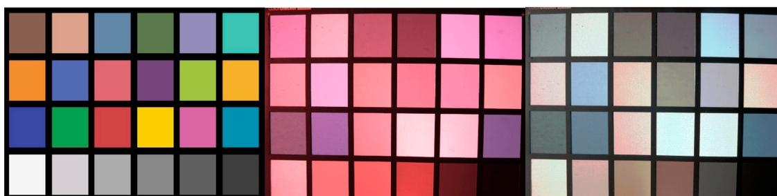
**Figure 3.** Macbeth Gretag color checker. (Left): original image in visible wavelengths. (Center): image under red and infrared lights. (Right): after equalization, the three channels R (red), G (infrared over 700 nm, IR1) and B (infrared over 800 nm, IR2) are equilibrated in exposures.
