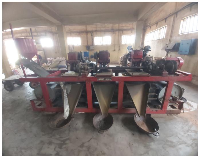
**Figure 4.** Rapid magnetic separator (source: National Metallurgical Development Centre (NMDC), Jos, Nigeria).
