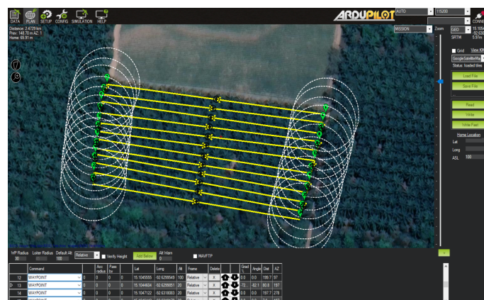
Figure 4. Palm crop flight plan created with Mission Planner software. The yellow lines indicate the UAV flight path and the green dots the waypoints.
