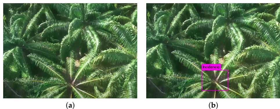
Figure 11. Detection of palms with BD. (a) False negative. (b) True Positive.
