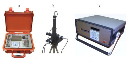
Figure 1. Recorder (a), magnetic sensors (b), and transmitter (c) of the CSRMT equipment.
