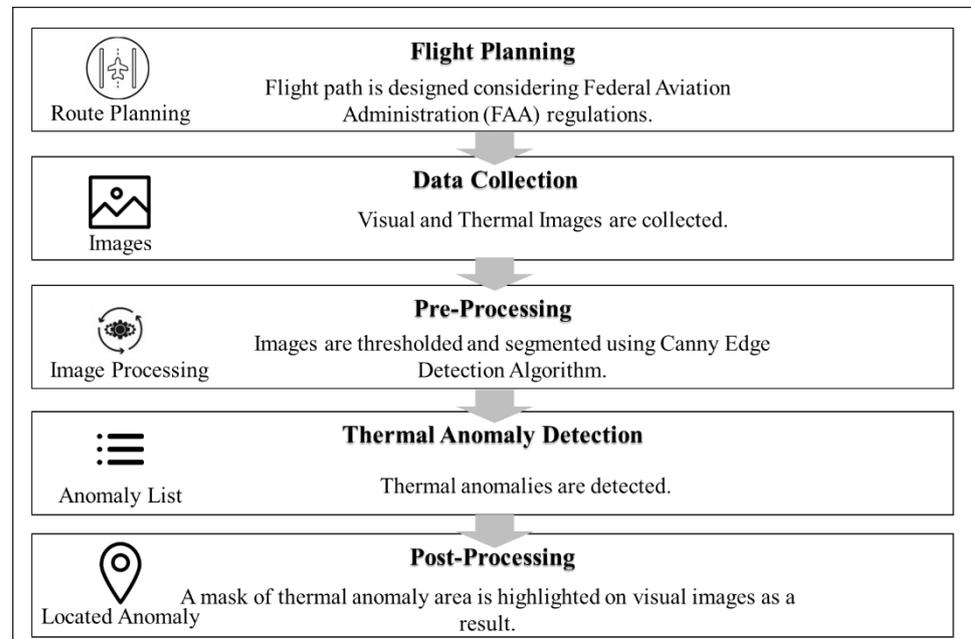
**Figure 14.** Energy assessment framework using UAS, proposed by [46].
