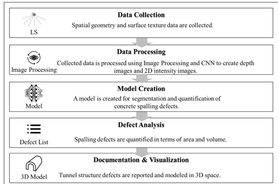
**Figure 10.** Concrete tunnel spalling inspection framework using LS, proposed by [31].
