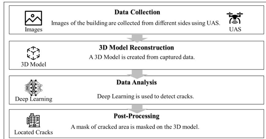
**Figure 12.** Building crack detection framework using UAS, proposed by [33].
