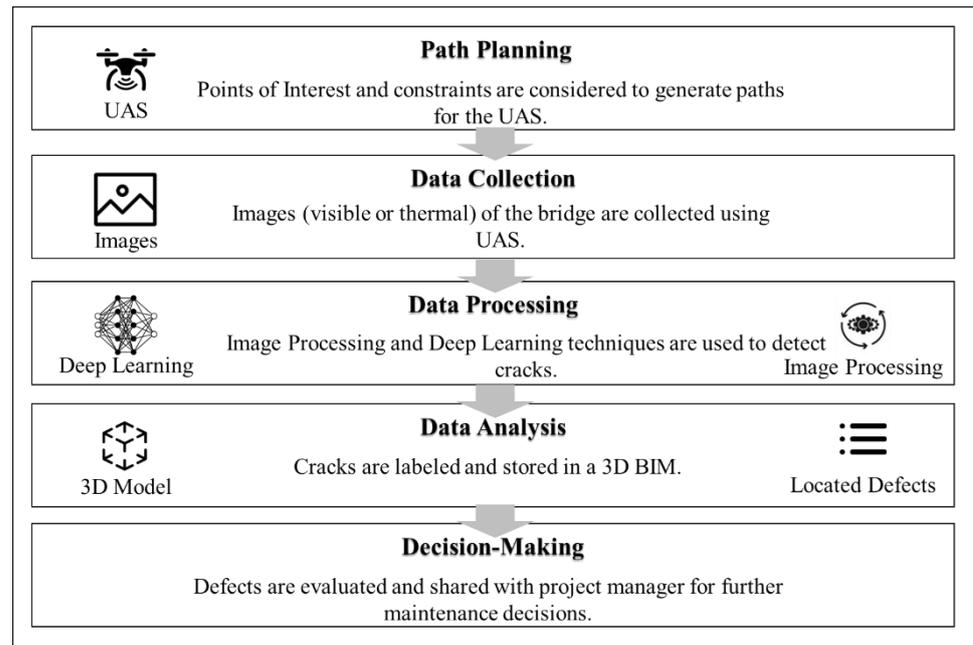
Figure 7. UAV-based bridge inspection framework, proposed by [23,24].
