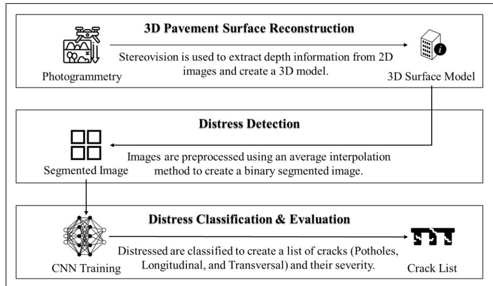
**Figure 4.** Automated 3D and CNN-based pavement inspection framework proposed by [10].
