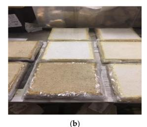
Figure 9. Drying test: (a) samples arranged during the test; (b) waterproofing of samples for unilateral drying.
