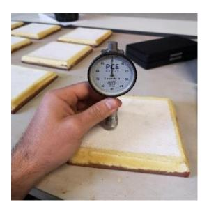
Figure 3. Surface hardness test with Shore A durometer.
