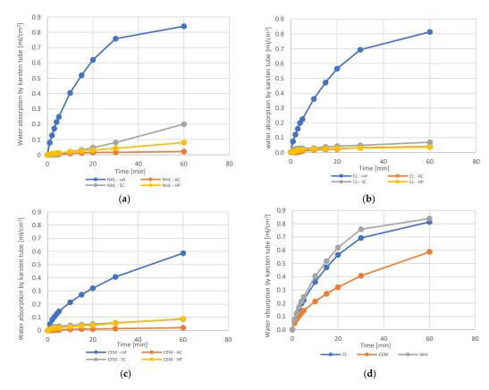
**Figure 13.** Water absorption curves for Karsten tubes: (a) curves related to NHL render; (b) curves related to CL render; (c) curves related to CEM render; (d) comparative curves of different renders without paint.
