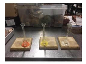
Figure 12. Absorption of water using the Karsten tube technique.
