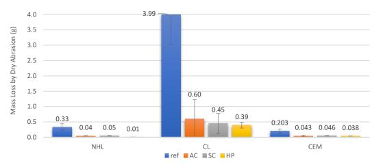
Figure 6. Mass loss through the dry abrasion resistance test.
