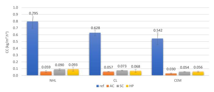
Figure 8. Coefficients of capillary water absorption.
