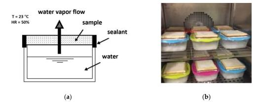
**Figure 15.** Water vapour permeability test: (**a**) schematic illustration of the capsule; (**b**) capsules inside the climatic chamber.
