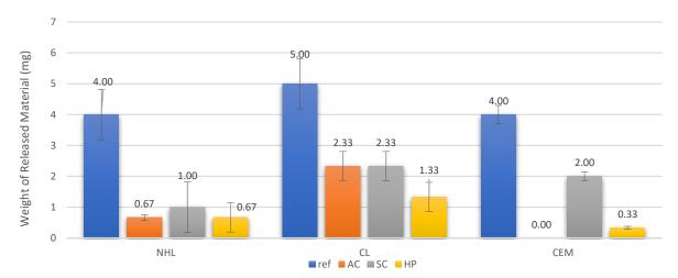
The results of the loss of surface cohesion obtained by the renders and corresponding paints studied are shown in Figure 5. These values were obtained by averaging the results of the three samples tested for each paint and render combination.
