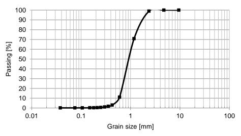
**Figure 1.** Aggregate particle size distribution curve.
