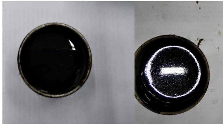
Figure 9. Penetration test samples of RB (left) and LP-15 (right).
