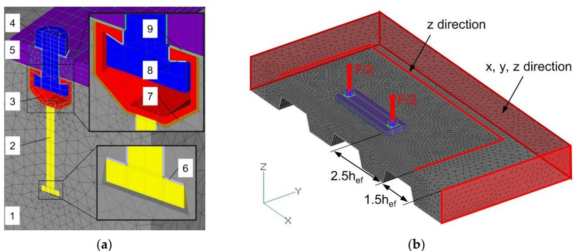
**Figure 3.** (a) FE discretization: 1—concrete slab, 2—anchor, 3—channel, 4—T-bolt with nut, 5—fixture, 6—anchor interface, 7—channel interface, 8—T-bolt interface, 9—PTFE sheet; (b) FE model and boundary conditions.
