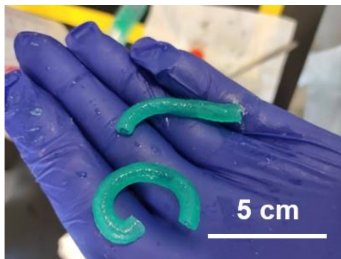
Figure 9. Alginate and Gelatin extruded ureters.
