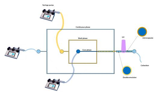
**Figure 3.** Microfluidic process to produce simple polymer microcapsules within situ UV polymerization of the shell.
