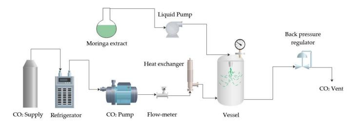
Figure 1. Schematic diagram of SAS 200 pilot plant.
