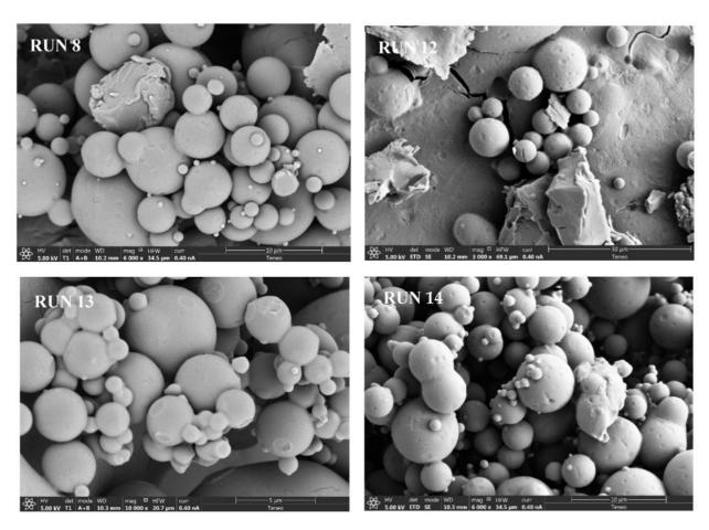
Figure 2. SEM images of Moringa-leaf particles precipitated using the SAE process.
