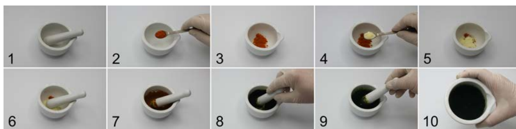
Figure 3. Mechanochemical preparation of Prussian blue from ferric chloride and potassium hexacyanoferrate(II).
