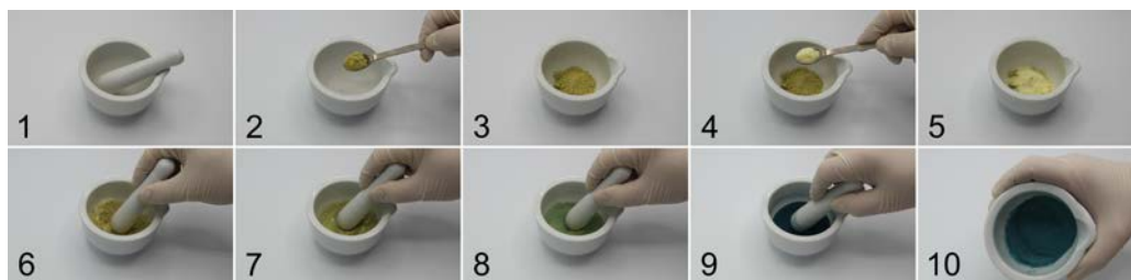
Figure 5. Mechanochemical preparation of Prussian blue from ferrous sulfate and potassium hexacyanoferrate(II).
