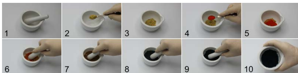
Figure 4. Mechanochemical preparation of Prussian blue from ferrous sulfate and potassium hexacyanoferrate(III).
