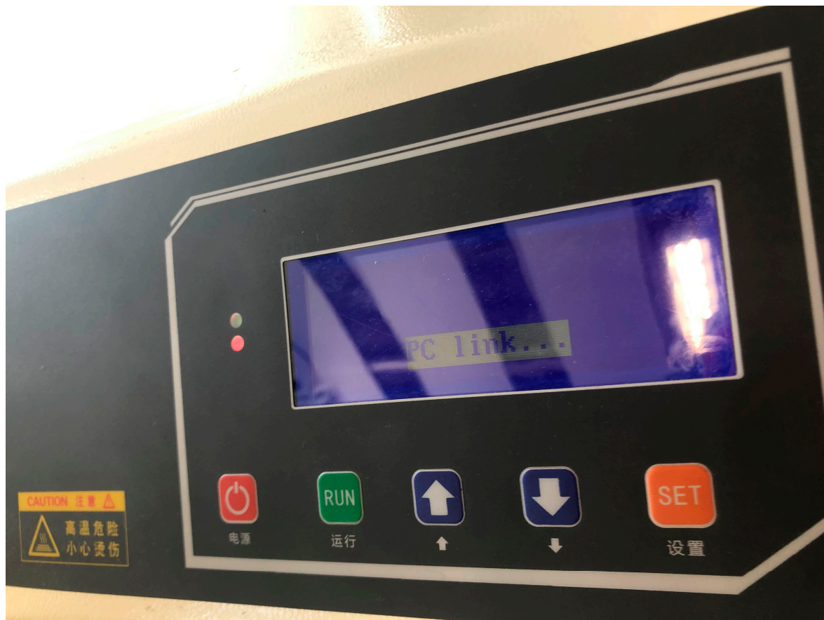
Figure 9. Reflow Oven’s Liquid Crystal Display (LCD) confirms successful “PC-link” mode entered. Red Light Emitting Diode (LED) to the left of the display indicates resistance is currently active and temperature increase is occurring.
