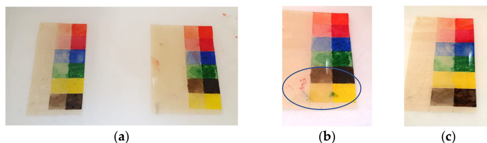
Figure 7. (a) Samples in a tub immersed in the solution, (b) untreated sample—color is unstable (see marked area), (c) sample treated with mucilage—color is stable.
