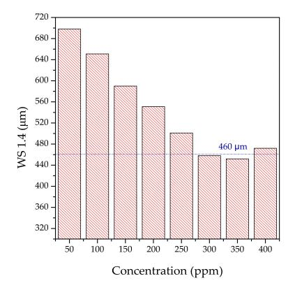
**Figure 8.** Impact of tobacco seed oil *N*,*N*-Bis(2-ethoxyethyl) amides addition on the lubrication characteristics of the base fuel.
