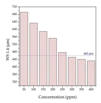
**Figure 2.** Impact of sunflower oil *N*,*N*-Bis(2-ethoxyethyl) amides addition on the lubrication characteristics of the base fuel.
