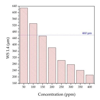
**Figure 6.** Impact of coconut oil *N*,*N*-Bis(2-ethoxyethyl) amides addition on the lubrication characteristics of the base fuel.
