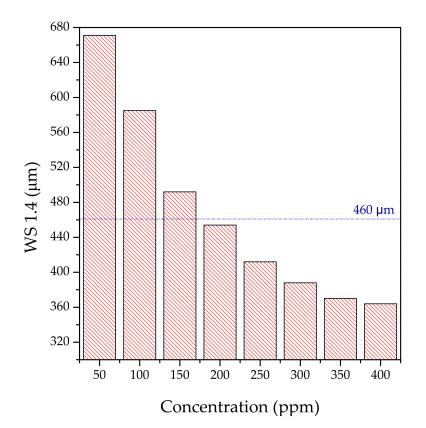
**Figure 4.** Impact of olive oil *N*,*N*-Bis(2-ethoxyethyl) amides addition on the lubrication characteristics of the base fuel.
