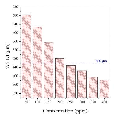
**Figure 7.** Impact of used frying oil *N*,*N*-Bis(2-ethoxyethyl) amides addition on the lubrication characteristics of the base fuel.
