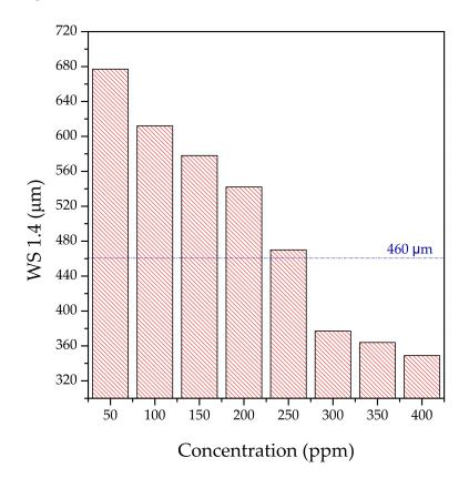
**Figure 5.** Impact of cottonseed oil *N*,*N*-Bis(2-ethoxyethyl) amides addition on the lubrication characteristics of the base fuel.
