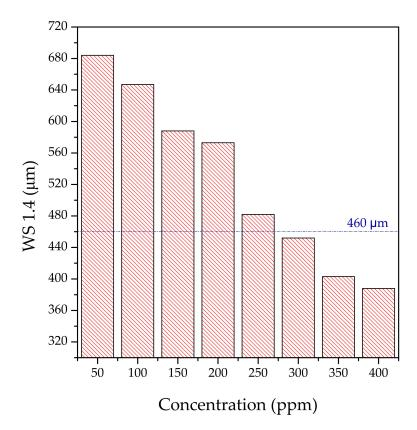
**Figure 3.** Impact of soybean oil *N*,*N*-Bis(2-ethoxyethyl) amides addition on the lubrication characteristics of the base fuel.
