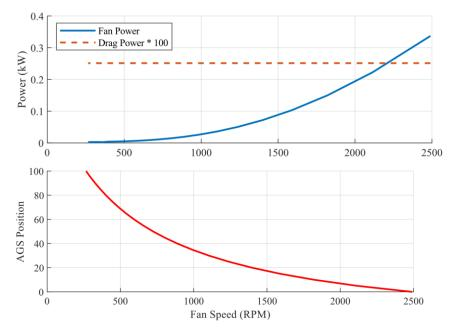
Figure 9. AGS position, fan speed, and power for 450 cfm airflow at 13.4 m/s vehicle speed.
