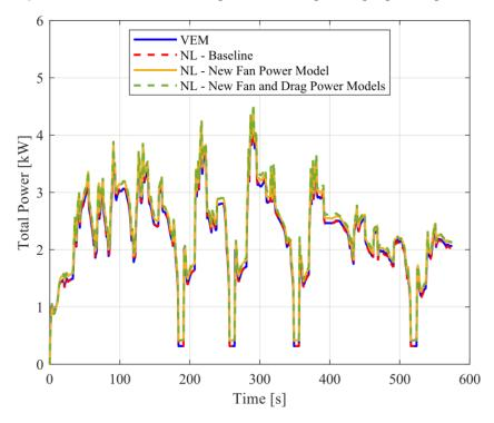
Figure 7. Total power consumption comparison for the SC03 drive cycle.
