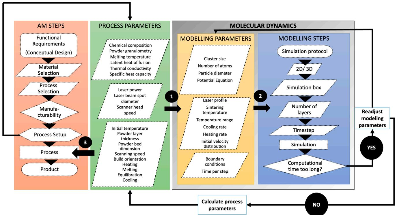
**Figure 2.** Flowchart of the framework, with process setup defining the process parameters, process parameters defining the modeling parameters (arrow number 1), modeling parameters defining the simulation protocol (arrow number 2), while final process parameters post-simulation defining the process (arrow number 3).
