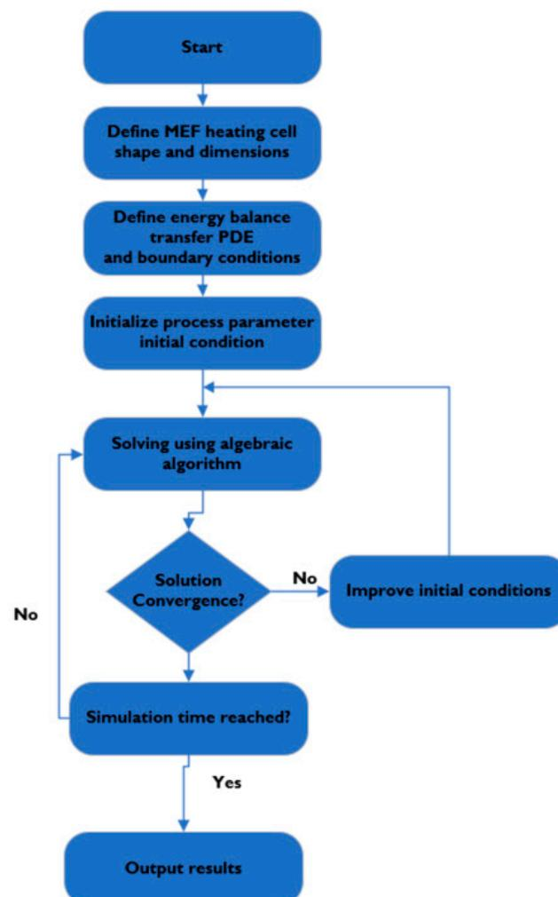
Figure 4. General procedure for numerical modelling and solving of PDEs.
