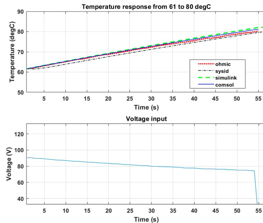
**Figure 19.** Model comparison between 61 and 80 °C.
