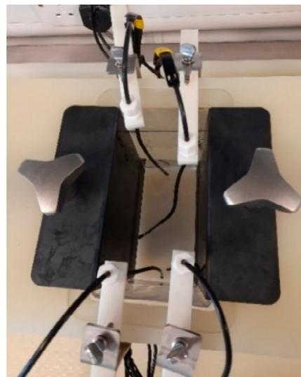
**Figure 16.** Heating chamber consisting of the heating cell, Ti electrodes, and 4 mounted thermocouples.
