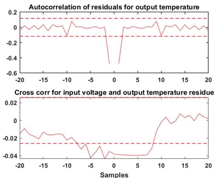
**Figure 14.** Plot of the correlation and residual analyses of the Discrete ARX (arx728) model.
