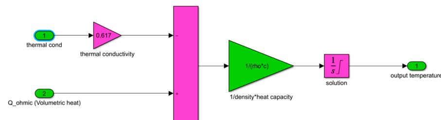
Figure 7. A snapshot of the heat determination block subsystem showing the energy balance equation ( $\rho c \frac{\partial T}{\partial t} = \nabla \cdot (k \cdot \nabla T) + Q_h$ ) and the integral used to determine its solution.
