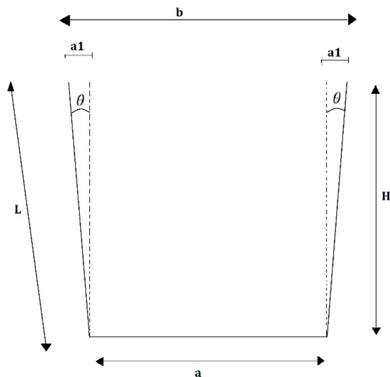
Figure 2. Modelling of the electric field between the slant electrodes of the batch Ohmic heater.
