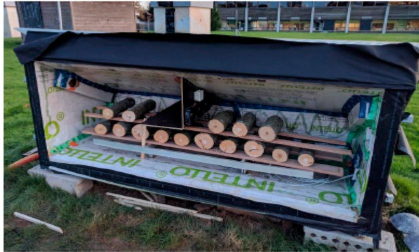
**Figure 2.** Drying chamber equipped with sensors and logs of wood to dry.
