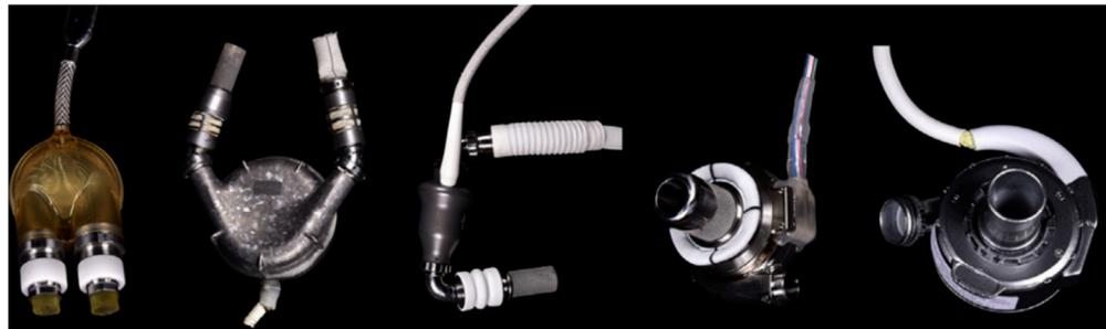
**Figure 1.** Implantable Mechanical Circulatory Support Devices. An example of clinically used ventricular assist devices from first, second and third generations. From left to right: PVAD, HeartMate XVE, HeartMate II, HVAD and the HeartMate 3. Image obtained with permission and modified from Elsevier and Kim et al., 2018 [14].
