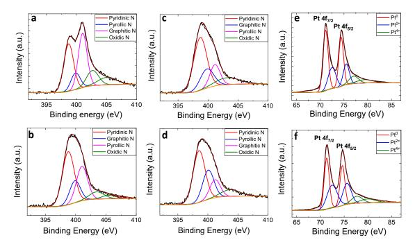
**Figure 2.** N 1s XPS spectra of (**a**) bare VACNF, (**b**) N-VACNF PA 5 min, (**c**) N-VACNF PA 15 min, and (**d**) N-VACNF PA 30 min; Pt 4f XPS spectra for (**e**) Pt/N-VACNF and (**f**) Pt/C.
