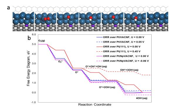
**Figure 5.** (a) Molecular structures of the most stable ORR intermediates over  $Pt/N_pVACNF$ ; (b) Free energy diagram of the 4-e<sup>-</sup> pathway for ORR on  $Pt/N_pVACNF$  (pink) compared with Pt (111) (red) and Pt/VACNF (blue) by both associative (dotted) and dissociative (solid) mechanisms. Color code: blue-Pt, gray-C, purple-N, red-O, white-H.
