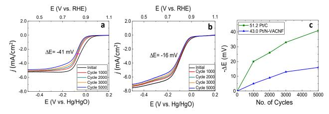
**Figure 6.** LSV curves of (a) Pt/C (51.2  $\mu$ g/cm<sup>2</sup>) and (b) Pt/N-VACNF (43.0  $\mu$ g/cm<sup>2</sup>) after every 1000 AST cycles in O<sub>2</sub>-saturated 0.10 M KOH solution at a scan rate of 10 mV/s and a rotation speed of 1600 rpm; (c) Change in the half-wave potential of the LSV curves vs. the number of AST cycles for all the catalysts.
