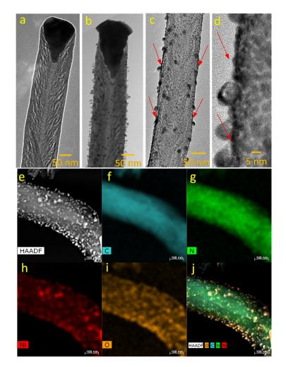
**Figure 1.** TEM image of bare VACNF (**a**) before and (**b**) after plasma annealing for 5 min at 550 °C. TEM image of Pt/N-VACNF PA 5 min (43.0  $\mu$ g/cm<sup>2</sup>) at (**c**) low and (**d**) high magnification. The red arrow indicates the Pt NPs deposited on the sidewalls; (**e**) HAADF-STEM image and (**f**–**j**) STEM-EDS elemental mapping of N-VACNF PA 15 min.
