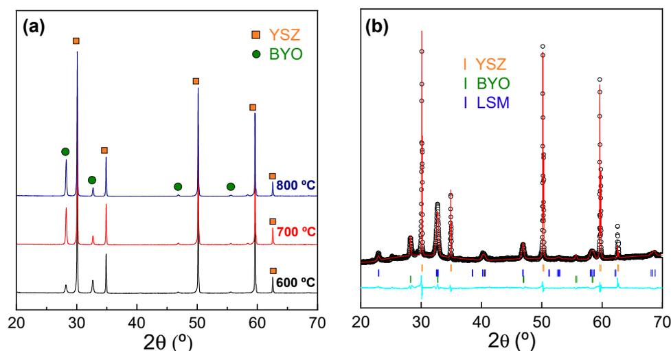
**Figure 1.** X-ray diffraction patterns of (a) Bi<sub>1.5</sub>Y<sub>0.5</sub>O<sub>3</sub> (BYO) films deposited on Zr<sub>0.84</sub>Y<sub>0.16</sub>O<sub>1.92</sub> (YSZ) substrates after calcining at different temperatures, and (b) Rietveld analysis of La<sub>0.8</sub>Sr<sub>0.2</sub>MnO<sub>3</sub> cathode deposited on BYO layer (SP-BYO/LSM).
