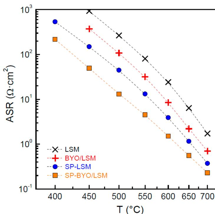
**Figure 6.** Area specific resistance (ASR) values of the different LSM cathodes as a function of the temperature.
