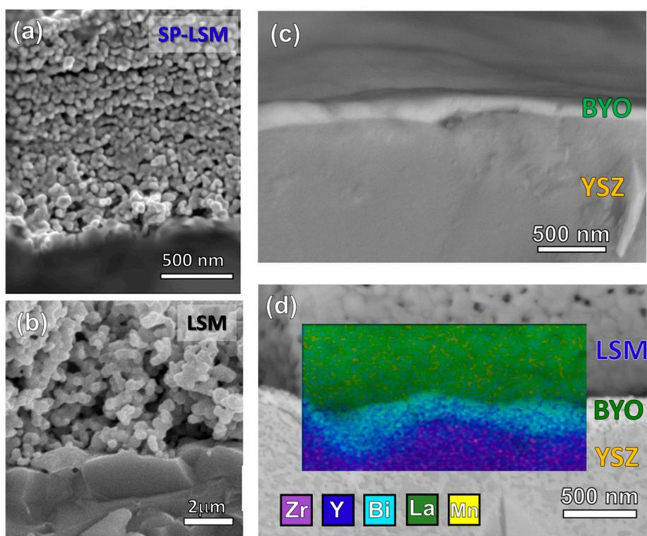
**Figure 2.** SEM image of (a) LSM cathode prepared by spray-pyrolysis; (b) LSM cathode prepared by screen-printing; (c) backscattering SEM, showing the dense BYO film deposited on the YSZ electrolyte; and (d) EDS mapping analysis of the different layers of the cells.
