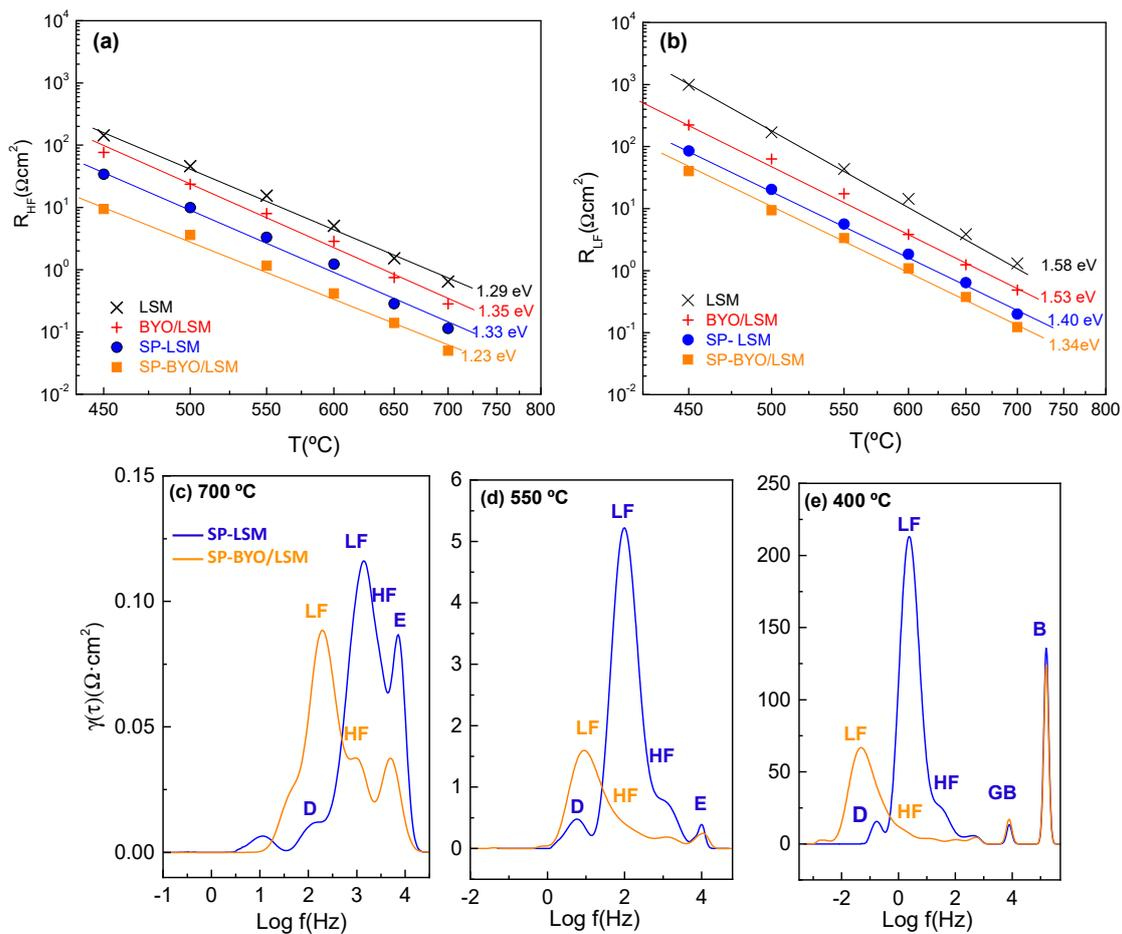
**Figure 4.** Variation of the (a) high- and (b) low-frequency resistance contributions for the different cathode configurations; (c–e) Distribution of relaxation time (DRT) analysis at different temperatures.
