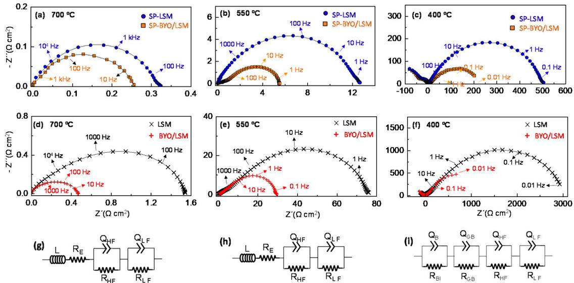
**Figure 3.** Impedance spectra of LSM and BYO/LSM symmetrical cells with LSM prepared by (a–c) spray-pyrolysis and (d–f) screen-printing at different measuring temperatures. (g–i) Equivalent circuits used to fit the data. The solid lines in the spectra represent the fitting curve with the proposed equivalent circuits.
