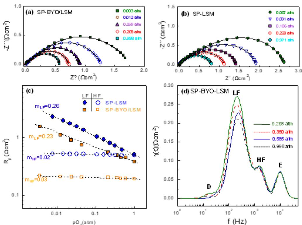
**Figure 5.** Impedance spectra of (a) SP-BYO/LSM; (b) SP-LSM at 650 °C and different  $pO_2$ ; (c) dependence of the cathode resistance contributions on  $pO_2$ ; and (d) the DRT analysis of SP-BYO/LSM.
