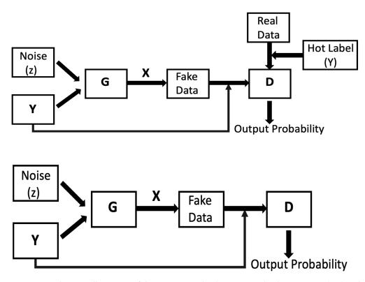
**Figure 4.** A schematic illustration of the process involved in training the discriminator (**top**) and the generator (**bottom**).
