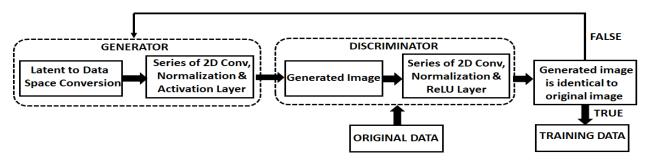
Figure 2. An overview of the scheme used to implement the cGAN to create new instances.
