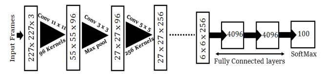
Figure 5. The AlexNet classification model used for the validation of our created dataset.
