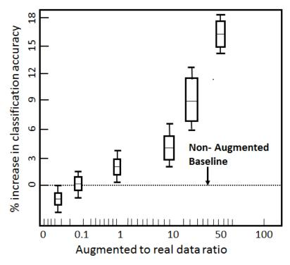
Figure 8. Impact of augmented-to-real data ratio on the classifier's performance.
