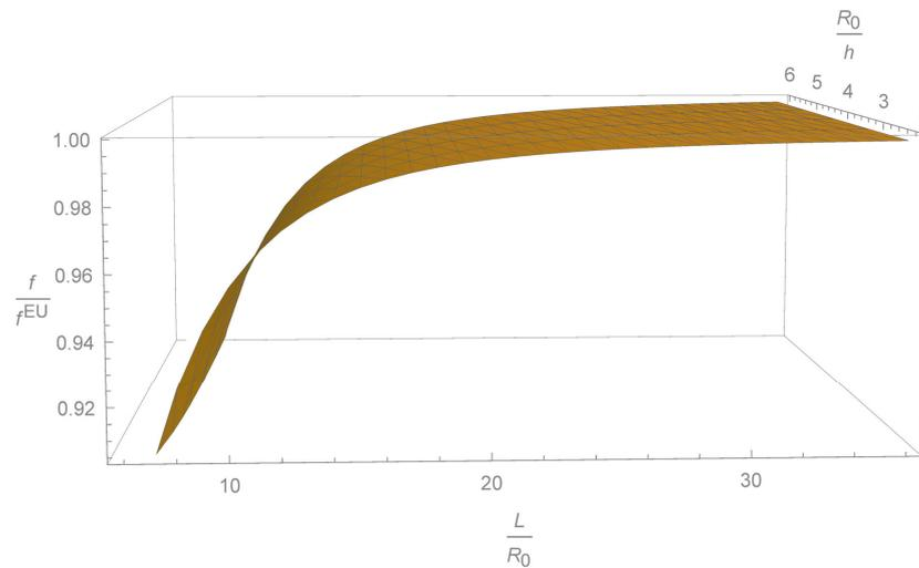
**Figure 4.** Plot of normalized natural frequencies vs. aspect ratios, with  $R_0/h = 6$  and two nonlocal parameter values  $\eta = 0, \eta = 0.2$ .
