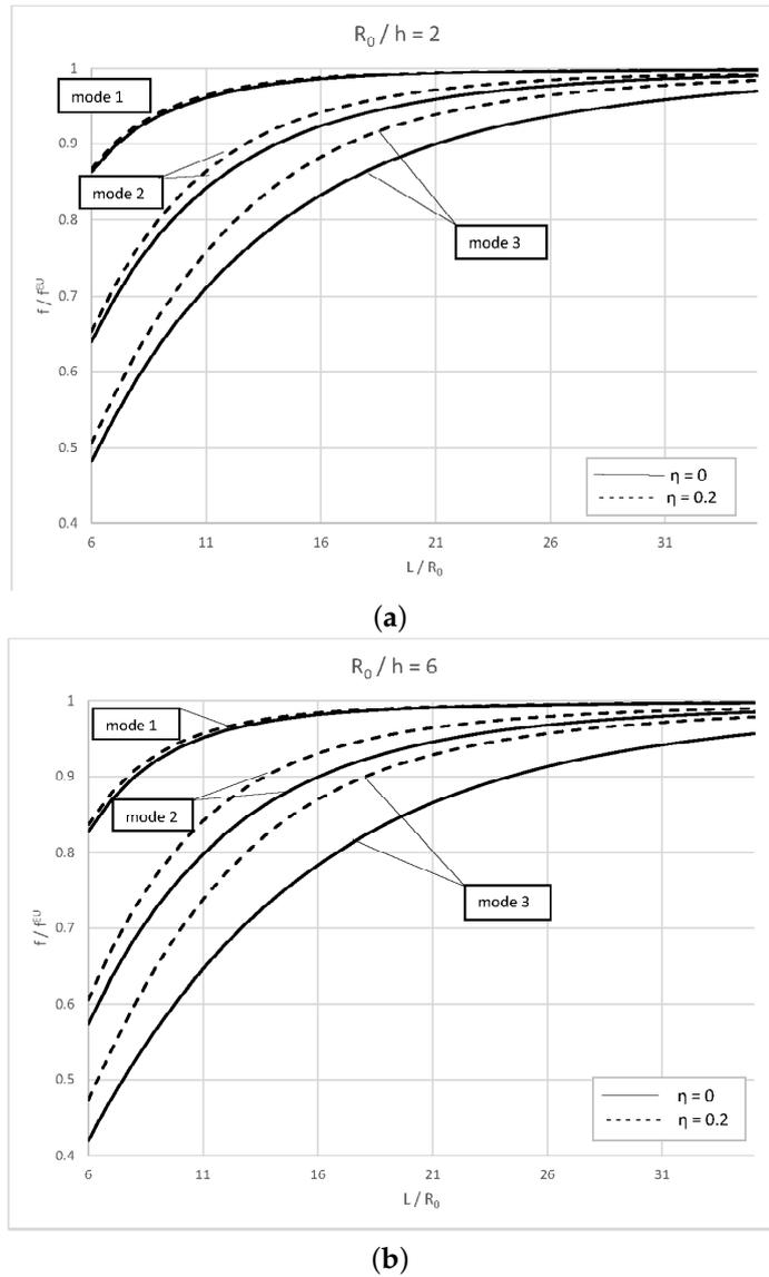
**Figure 3.** (a) Plot of normalized natural frequencies vs. aspect ratios, with  $R_0/h = 2$  and two nonlocal parameter values  $\eta = 0, \eta = 0.2$ ; (b) Plot of normalized natural frequencies vs. aspect ratios, with  $R_0/h = 6$  and two nonlocal parameter values  $\eta = 0, \eta = 0.2$ .
