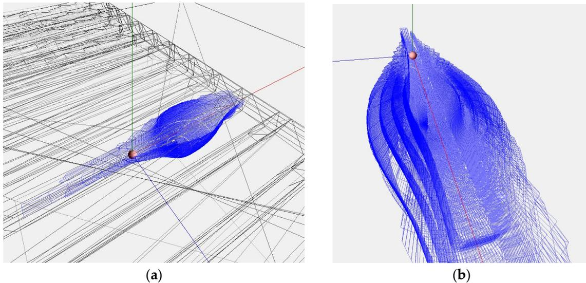
**Figure 3.** Example of forming the outline of the elastic wave front in the ballast layer: (a) at one time step; and (b) changing the outline with steps.
