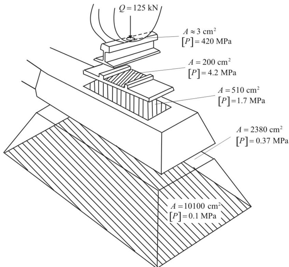
**Figure 2.** The load distribution in the railway superstructure on the basis of [8,15].
