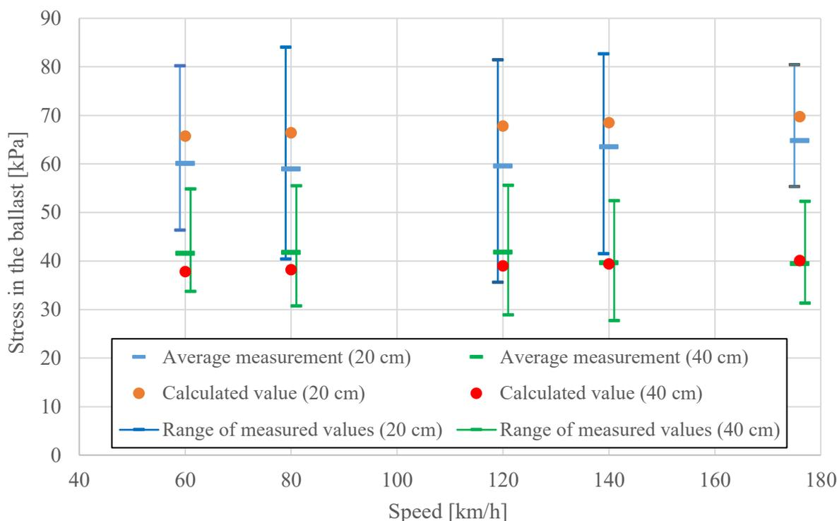
Figure 5. Comparison of experimental and calculated stresses in ballast.
