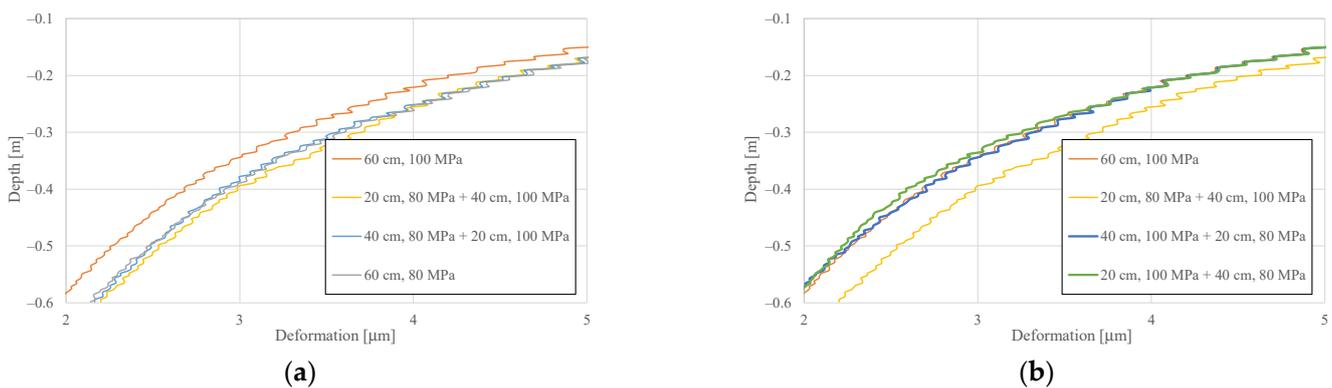
**Figure 6.** Deformation gradient of the ballast layer: (a) penetration of pollutants at different depths; and (b) varying position of the contaminated zone. The depth values are determined from the bottom surface of the sleeper; its height is  $\pm 0.0$  cm.
