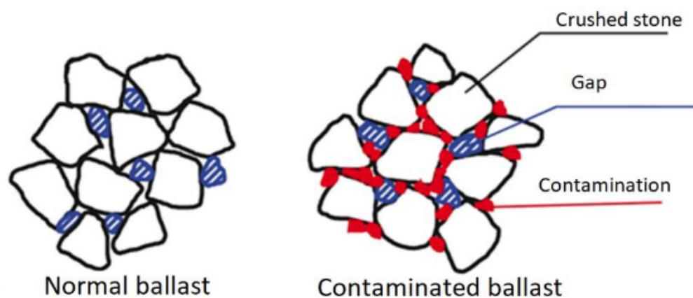
**Figure 1.** The contamination of the ballast based on [8].
