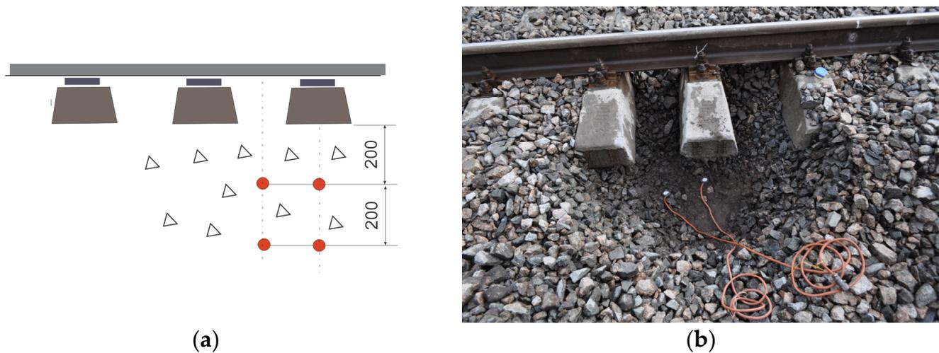
**Figure 4.** Placing mesoscopes (strain gauges) in the ballast layer: (a) installation scheme (the units are in mm); and (b) experimental site.
