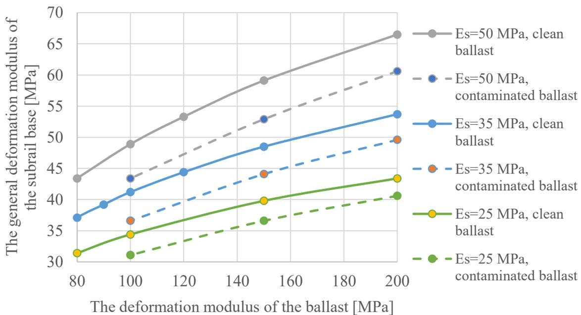
Figure 8. Dependence of the general deformation modulus of the sub-rail base on the characteristics of the ballast and soil.
