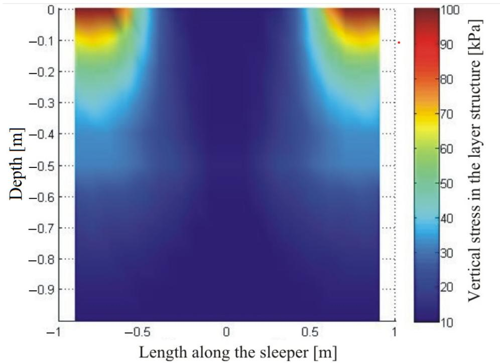
Figure 7. Propagation of stresses in the sub-sleeper layer in cross-section.
