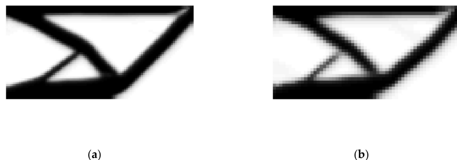
Figure 11. Cantilever with a load in the corner: final topologies using uniform grids of (a) 100 \times 50 and (b) 60 \times 30 bilinear finite elements.
