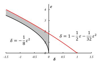
**Figure 1.** Ince–Strutt stability diagram for the Mathieu equation. The shaded region represents the domain of stable solutions for a tensile-loaded beam.
