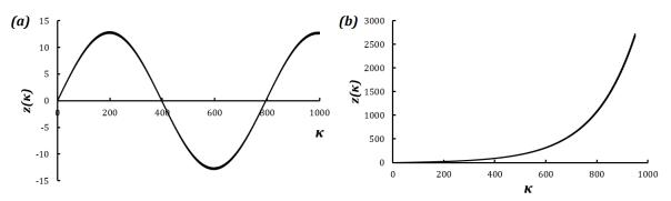
**Figure 2.** Solutions to the Mathieu equation for a tensile loaded beam with boundary conditions z = 0 at  $\kappa = 0$  and  $dz/d\kappa = 0$  at  $\kappa = 0$ . (a) Stable solution for  $\delta = -0.00025$ ,  $\varepsilon = 0.05$ , and (b) unstable solution for  $\delta = -0.00035$ ,  $\varepsilon = 0.05$ .
