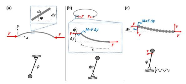
**Figure 3.** The deflection of a beam due to (**a**) compressive load F (corresponding to the stable equilibrium of a regular pendulum), and (**b**) tensile load F (corresponding to the unstable equilibrium of an inverted pendulum). (**c**) The waviness of the beam would stabilize the equilibrium similarly to the vibrations stabilizing an inverted pendulum (reproduced with permission from [11]).
