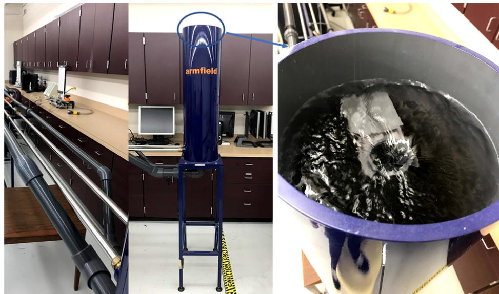
Figure 2. Laboratory water hammer system [1].
