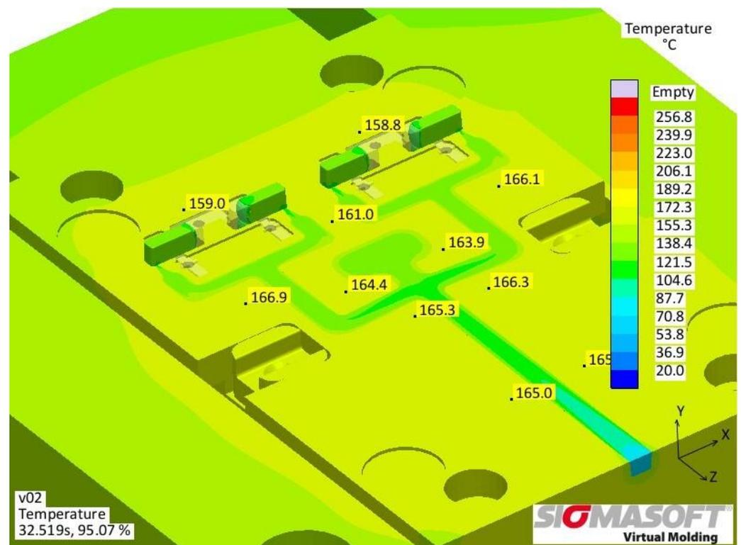
Figure 5. Filling simulation in sigmasoft.
