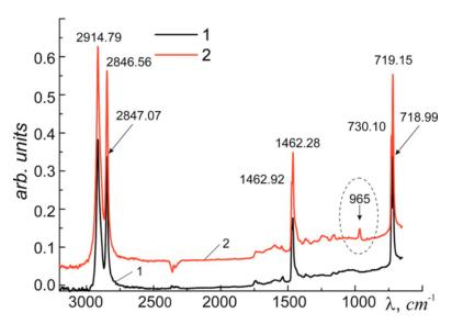
**Figure 3.** IR spectra of UHMWPE before (black—1) and after (red—2) treatment in helium plasma at low pressure (discharge power 50 W, helium flow5 cm<sup>3</sup>/min).
