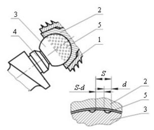
**Figure 2.** The scheme of texturing the surface of the femoral head in order to reduce the wear of the polymer liner: 1. Femoral head; 2. Polymer liner; 3. Cup; 4. Stem; 5. Lubrication layer.
