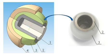
**Figure 4.** General view and 3D-model of a cup with a modular head obtained using the technology of soldering alumina ceramics with a titanium alloy: 1. Tapered neck of a total hip joint endoprosthesis stem; 2. Titanium alloy blind hole sleeve; 3. Alumina ceramic femoral head; 4. Cup.
