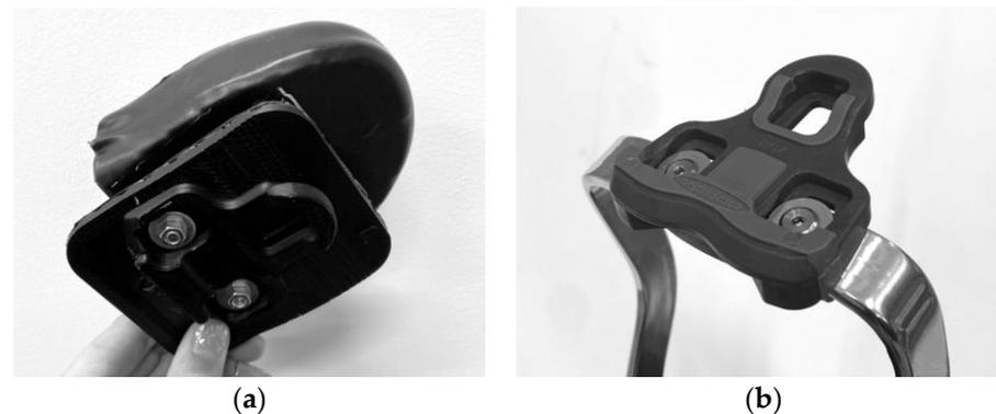
**Figure 6.** (a) 3D printed platform and its fitting compared to (b) a regular cycling cleat.
