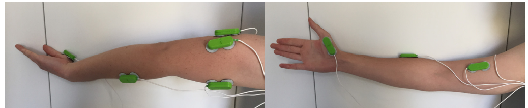
Figure 2. Photographs of the positions of EMG sensors (green boxes) on an anonymised participant. The left image shows the frontal plane of the arm. The right image shows the arm internally rotated to provide a view on the sensors placed on the triceps. In order to be representative of a prosthetic use case, the sensor placed on the hand was not used.
