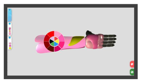
**Figure 2.** Developed customization web portal for selecting different 3D geometries and color palette selection, with full 3D visualization and manipulation.
