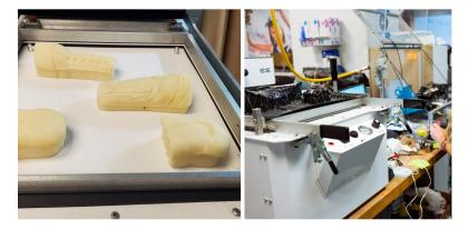
**Figure 1.** (Left side) A converted positive mold or "buck" for thermoforming application. (**Right** side) is thermoformed parts produced from a single sheet of ABS plastic, prepared for trimming.
