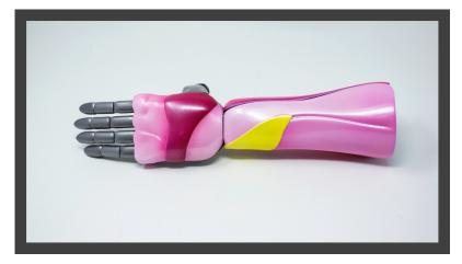
Figure 4. Completed aesthetic cosmesis components assembled on prosthesis for clinical investigation.
