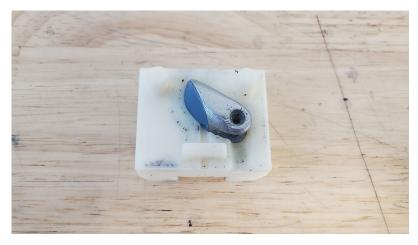
**Figure 5.** Overmolding achieved on additive manufactured component moulded using a silicon elastomer in a chamber produced by additive manufacturing.
