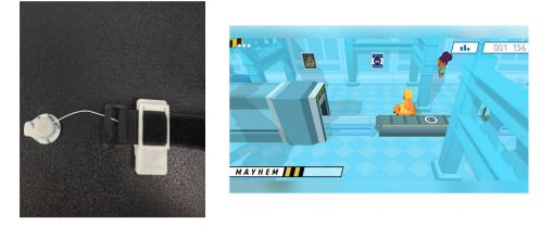
**Figure 6.** (Left side) Three-dimensional printed housing for electromyographic game controller, with interface surface electrode stickers and restraint. (**Right side**) In-game image of "Limbitless Runner" training game.
