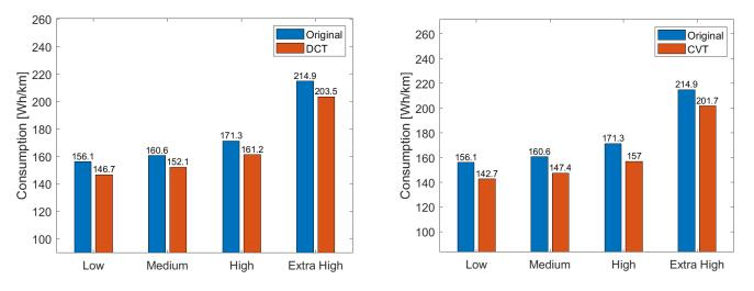
**Figure 19.** Comparison between the energy consumption of the original transmission and DCT (**left**) and CVT (**right**) for vehicle T in the four different phases of the WLTC cycle.
