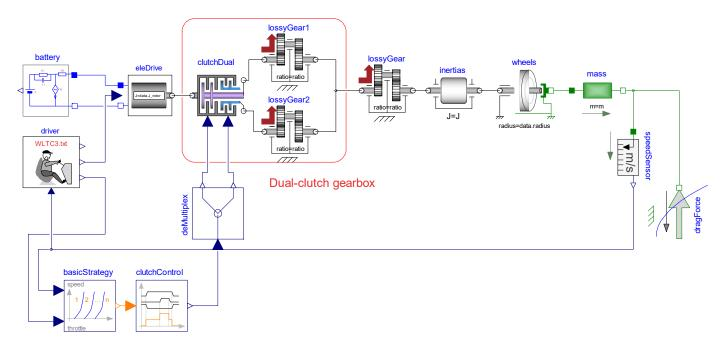
Figure 7. Diagram of the two-speed BEV simulation model.
