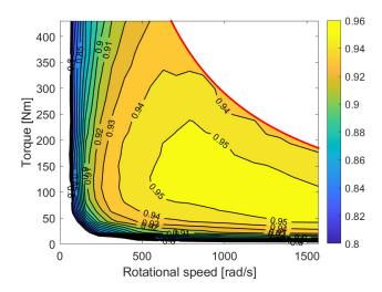
Figure 3. Vehicle T's electric drive efficiency map.
