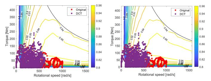
**Figure 17.** Comparison between the operating points of the original gear ratio and DCT (**left**) and CVT (**right**) on the electric drive efficiency map for vehicle T.
