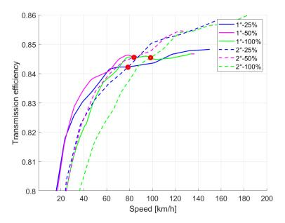
Figure 11. Transmission efficiency for the two gears selected for vehicle N.
