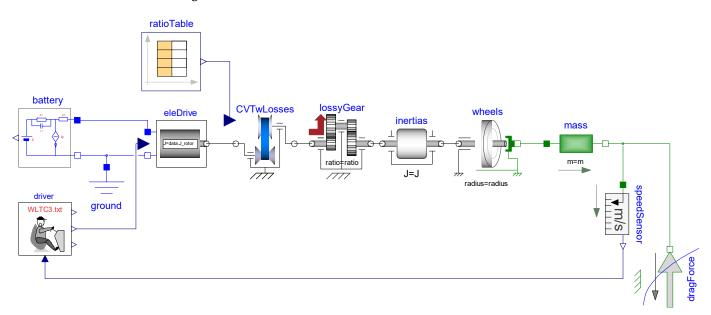
Figure 15. Diagram of the CVT BEV simulation model.
