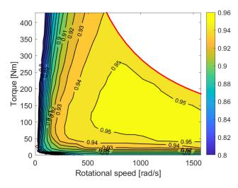
Figure 2. Vehicle T's motor efficiency map.
