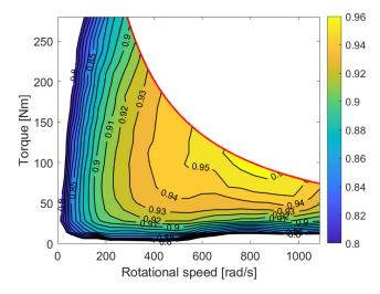
Figure 1. Vehicle N's electric drive efficiency map.
