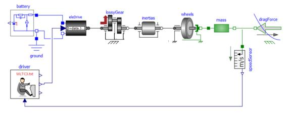
Figure 4. Diagram of the single-speed BEV simulation model.
