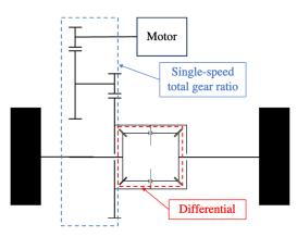
Figure 6. Schematic of a single-speed gear.
