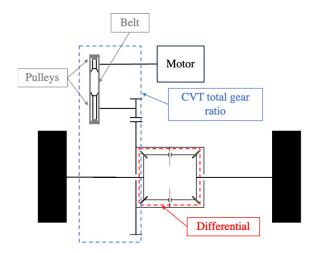
Figure 14. Schematic of CVT.
