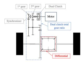
Figure 8. Schematic of the dual-clutch transmission.
