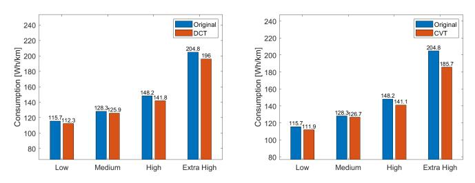
**Figure 20.** Comparison between the energy consumption of the original transmission and DCT (**left**) and CVT (**right**) for vehicle N in the four different phases of the WLTC cycle.
