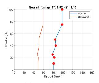
Figure 13. Vehicle N's gearshift map.
