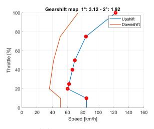
Figure 12. Vehicle T's gearshift map.
