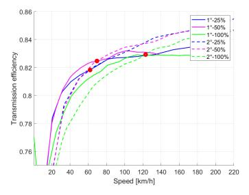
Figure 10. Transmission efficiency for the two gears selected for vehicle T.
